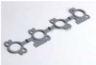
Molykote 7620, roll-coated on exhaust manifold gaskets, eliminates stick-slip between dissimilar metal parts and improves sealing properties.
