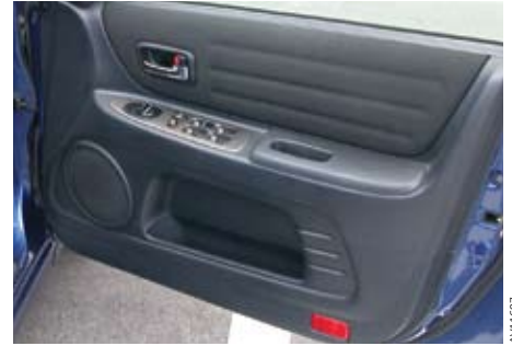
Molykote D-96, when used as a replacement for non-woven tape, eliminates squeaks and rattles in door trim assemblies.
